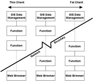
FIGURE 3 – Thin Client versus Fat Client Function Assignment
