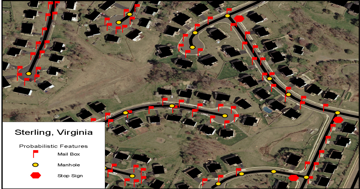
Figure 3. An aerial photo of a suburban setting overlaid with existing geospatial data (building footprints and street centerlines in black) and predicted positions of probabilistic features (residential mailboxes, and stop signs in red and manholes in yellow.) Image courtesy of http://seamless.usgs.gov .
