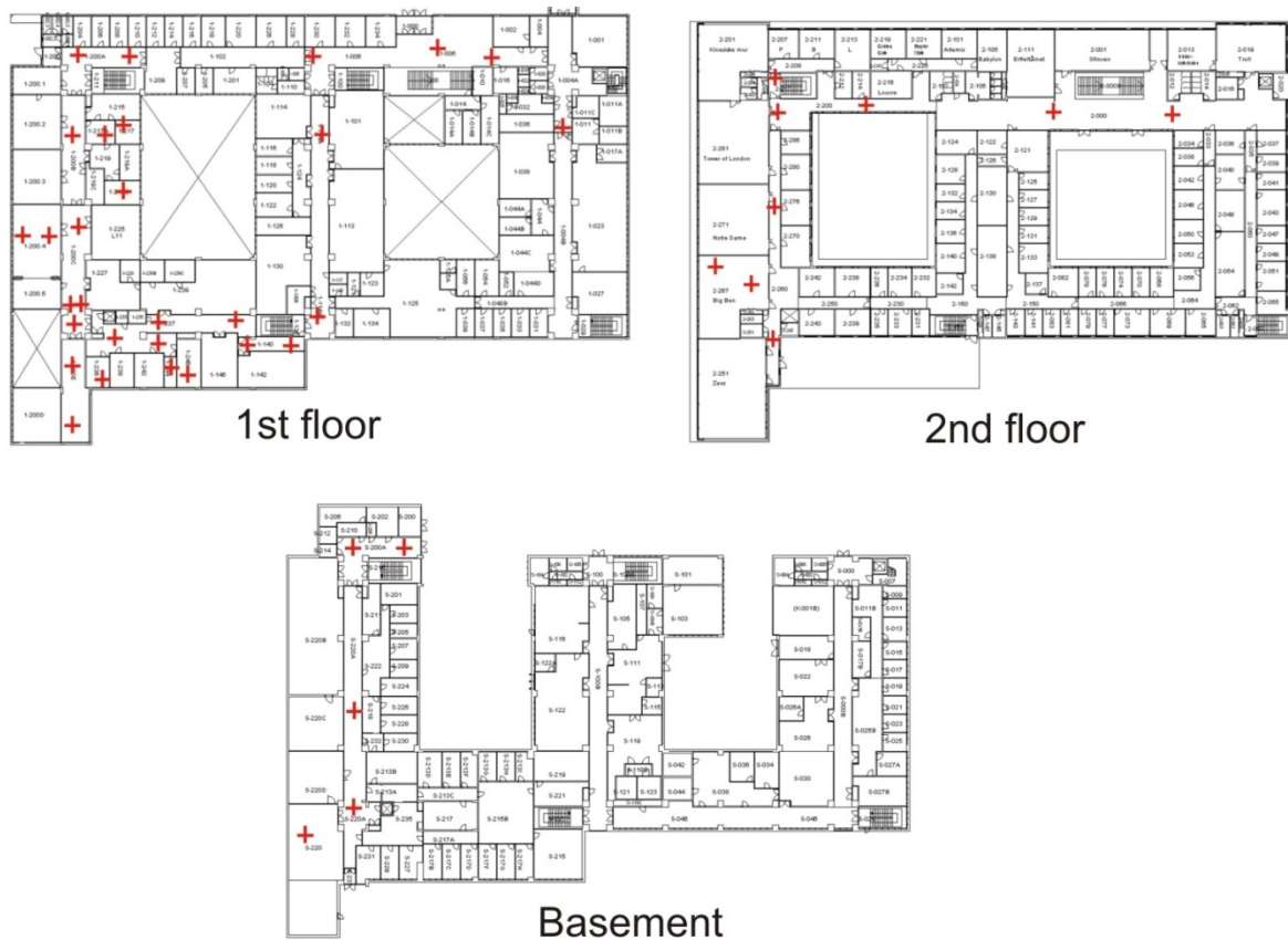
Figure 2: Control points established in the building.
