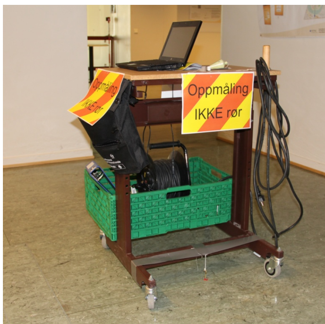
Figure 3: Movable platform for measuring control points.
