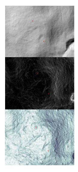
Figure 7: illustrates depressions in the three LiDAR models ranging from least visible (top image) to the most visible (bottom image). The red point is located in the approximate center of the feature.
