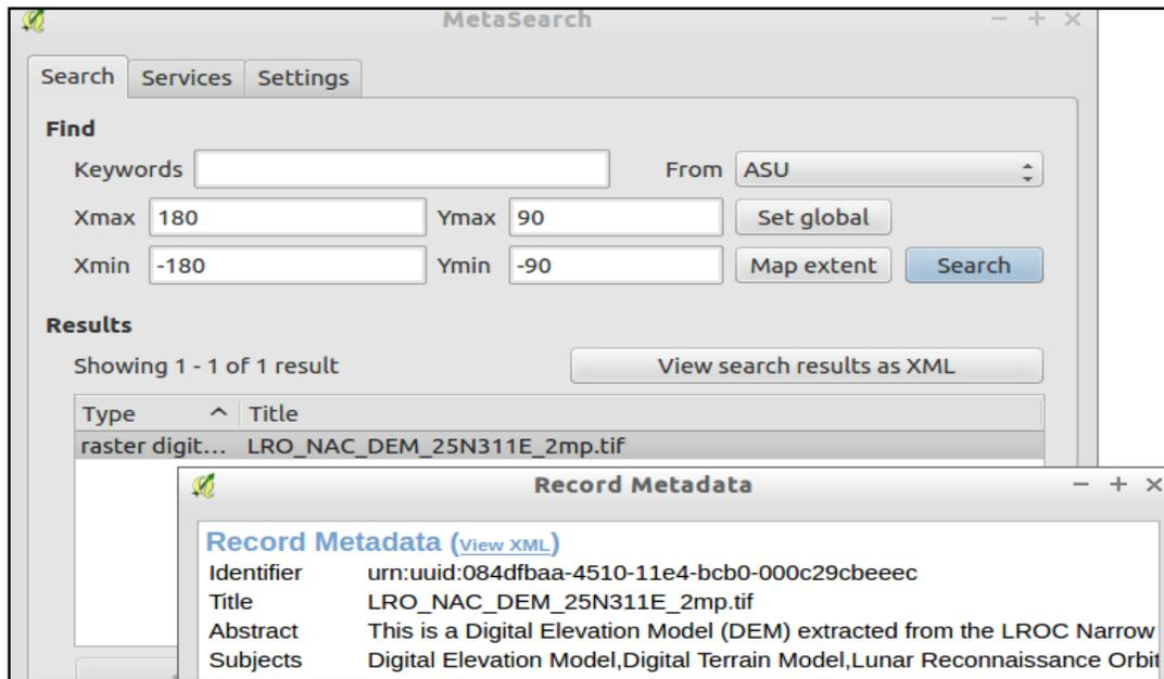
Figure 5: An example CSW search using the Desktop GIS application QGIS with a CSW plug-in. In this case, the CSW server returned a digital elevation model as derived from Lunar Reconnaissance Orbiter Camera images.
