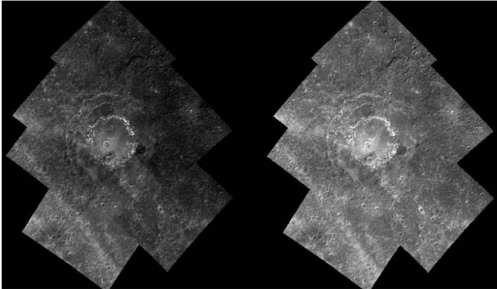
Figure 3: Example image mosaic of Raditladi crater (258 km diameter across) from NASA's Mercury Dual Imaging System (MDIS) on the MESSENGER spacecraft showing no photometric correction (left) and then the same image mosaic after applying the photometric corrections to the images prior to the mosaic creation (right). Image credit: NASA/USGS (K. Becker).
