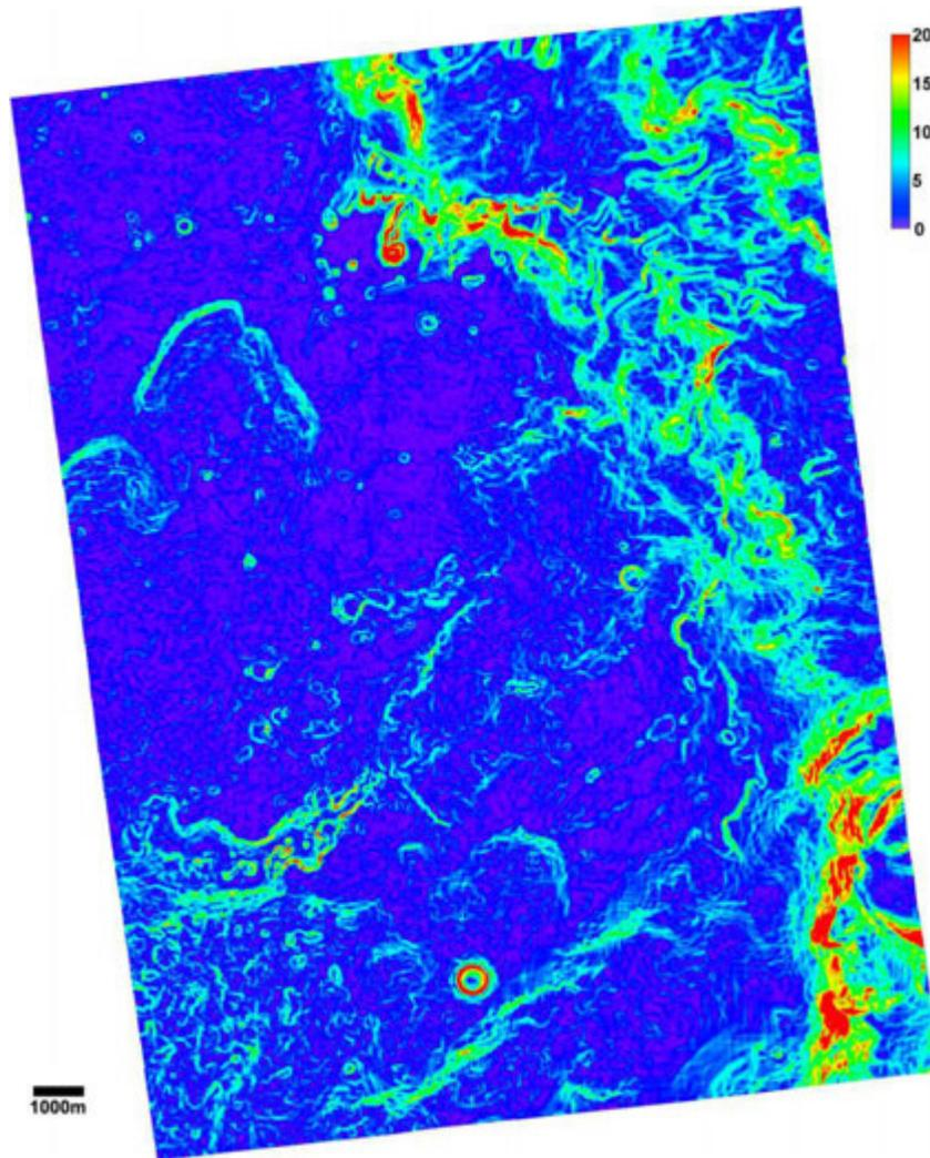
Figure 4: Example derived slope map at 20 meters/pixel within McLaughlin crater (center at 21.9° north 337.63° east) generated for the Mars 2020 rover mission. The slope map will be used to help assess the ability to land the rover safely on surface. Image credit: NASA/USGS.
