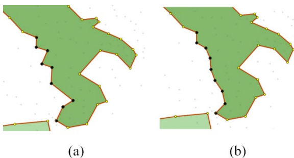
Figure 2. Application of a tool for automatically smoothing polygon vertices while preserving area. Figure shows a section of the Italian coastline after some local adjustments had created an unnatural jagged appearance: (a) before applying the smoothing tool and (b) after applying the smoothing tool.
