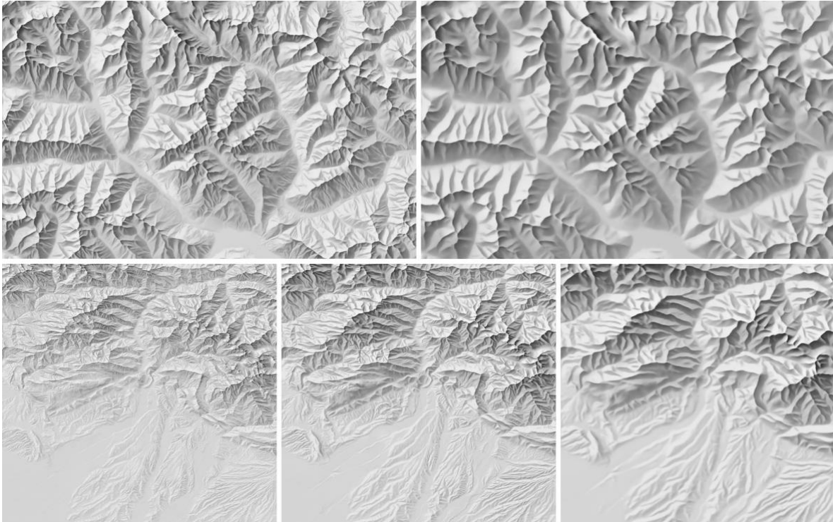
Figure 1: Adjusting the level of generalization by applying neural networks trained with reference elevation models with different cell sizes (top) and down-sampling and filtering input elevation models (bottom). Grossglockner, Austrian alps (top) and Zugdidi, Georgia (bottom). Relief shading with Eduard , an application for relief shading with neural networks ( https://eduard.earth ).
