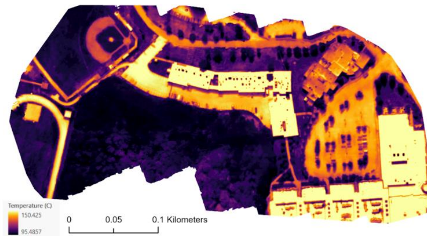
Figure 2: Thermal image orthomosaic constructed from images taken during a flight in Roanoke, VA using Mavic Pro Duo thermal camera, visualized with ironbow colormap
