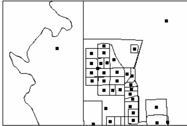
Figure 2. A portion of the analysis layer shown in Figure 1. A centroid has been calculated for each of the analysis features
