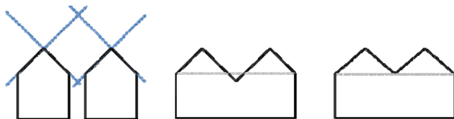
Figure 9. Front-view of two saddleback building models and their cell decomposition (dashed blue lines) and two possible aggregation results.
