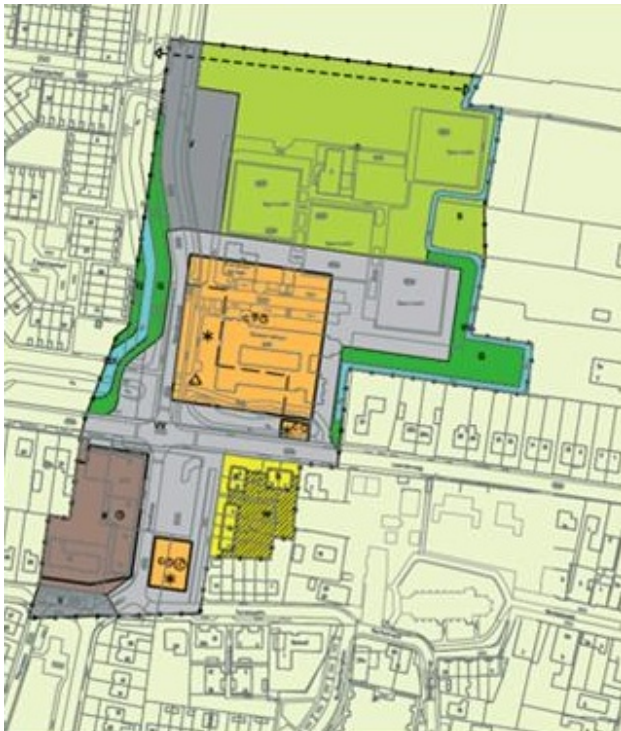
Figure 1. Example of a physical planning map with two layers: primary plan information, projected onto a topographic base map
