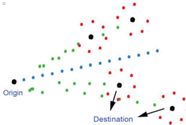
Figure 1 Candidate Nodes for Approximate Steiner Tree (red: points around destinations, green: points on the line segments from origin to destination, blue: external points)
