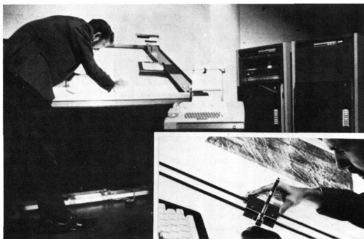
Figure 10.--Graphic digitizer and closeup of digitizer position.
