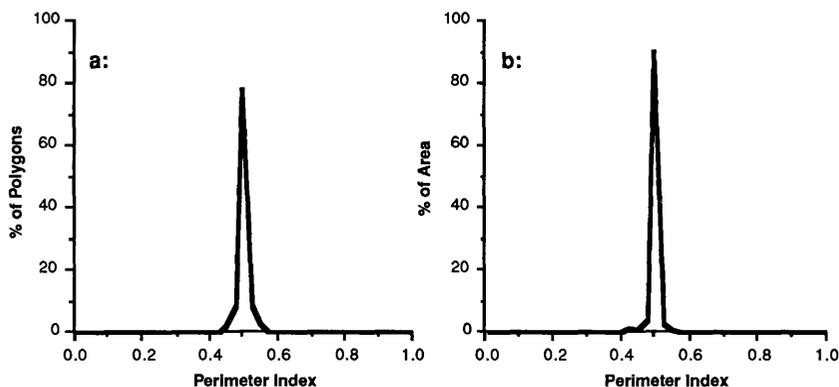
As Figure 7 shows, this purely positional error is closely packed around the theoretical value of 0.5. This indicates that the index correctly interprets the translation as a positional error.
