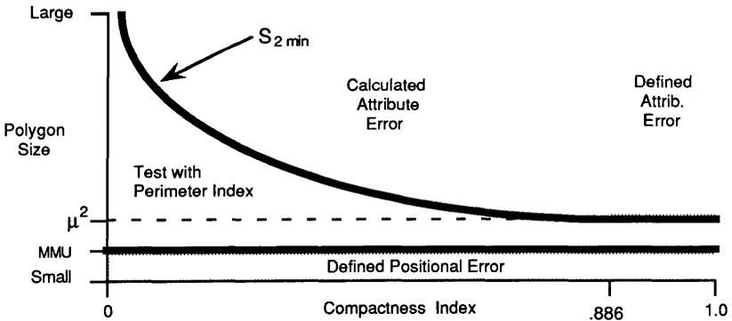
For the sixth and final stage of the test, a perimeter index is calculated for all polygons not previously classified. The perimeter index, discussed more fully below, is a ratio of the perimeter from one source to the total of the non-coincident perimeter from both sources. With this index, each remaining polygon falls into one of three categories: attribute, ambiguous (gray zone) or positional error.
