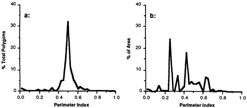
The pattern in Figure 4 (particularly part b) is somewhat clouded because it includes all polygons. While there is a central tendency between .4 and .6 in the number of polygons, much of the total map area comes from a few large polygons. The overlay generates 681 polygons, 106 of which are not errors. As shown in Map 3, these 106 polygons have 85.8% of the area, hence they dominate Figure 4b.
