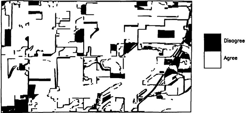
The areas of the polygons created by the overlay can be crosstabulated by the categories from the two source maps in the form of a matrix called a misclassification matrix by the Proposed Standard for Digital Cartographic Data Quality (Morrison, 1988, p.133), as in Table 1.
