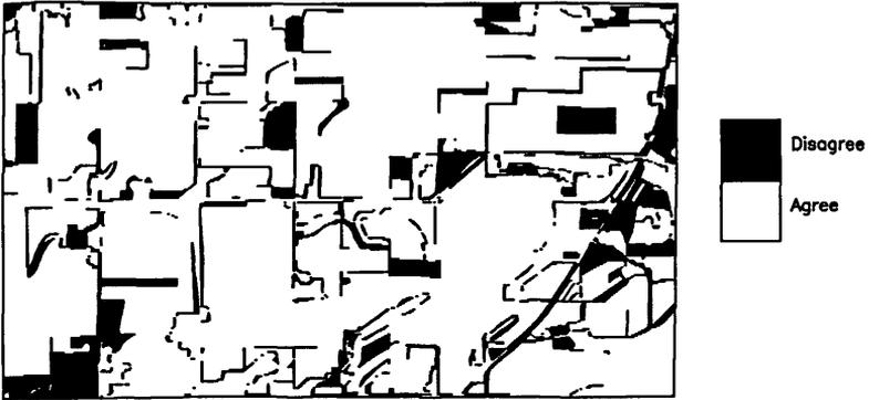
The areas of the polygons created by the overlay can be crosstabulated by the categories from the two source maps in the form of a matrix called a misclassification matrix by the Proposed Standard for Digital Cartographic Data Quality (Morrison, 1988, p.133), as in Table 1.
