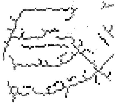
(7 b) Spots from Gaussian curvature detector in white. Linear segments attached to houses, to be deleted, in black.
