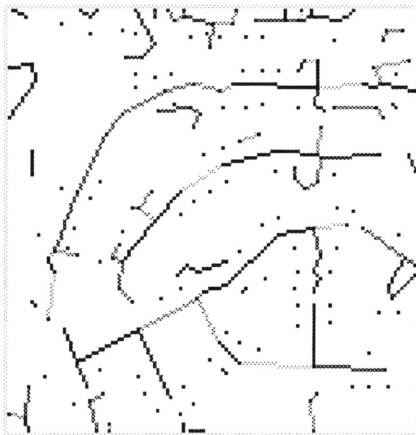
Figure 1b. Features located in CIRCLE. Straight line segments from roads are plotted different shades of gray. Isolated black dots are buildings.
