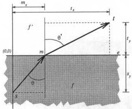
Fig. 27: Snell's Law of Refraction.
