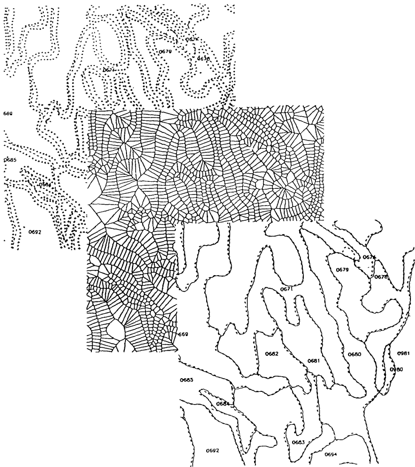
Fig. 1. a) Points digitized around the interior of each polygon; b) the Voronoi cells generated; c) the polygon boundaries generated (solid lines), compared with the original map (dashed lines).
