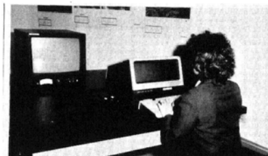
Figure 5. Digital Interactive Multi-Image Analysis System for semi-automated Landscape Feature Extraction from LANDSAT MSS Digital Imagery.
