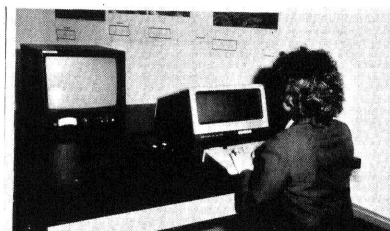
Figure 5. Digital Interactive Multi-Image Analysis System for semi-automated Landscape Feature Extraction from LANDSAT MSS Digital Imagery.
