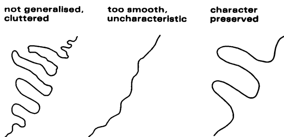
FIGURE 5--A severe change in scale might warrant the selective elimination of some features of a given type and the enlargement of others. For example, a reduction in the number of inlets not only prevents clutter but preserves the character of a fjorded coast. Merely smoothing the coastline yields a symbol with less information about the form of the coast and its geomorphic history.
